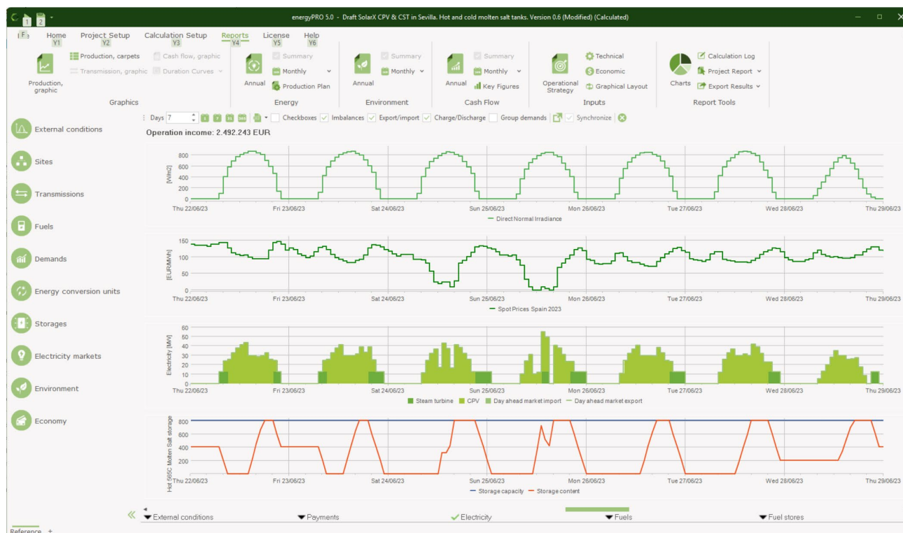
Figure 3 . Example: On 23 June 2023, salt storage (red curve at the bottom) charges during low day-ahead electricity prices (dark green curve); electricity is generated in the evening during peak prices.
