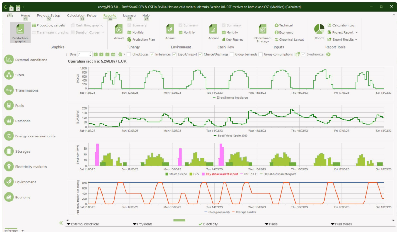
Figure 5. Example: On 14 March 2023, salt charging occurs at night via grid power; turbine operates in the morning.
