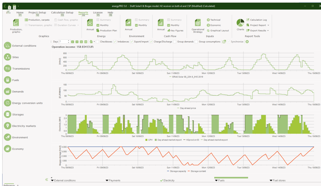
Figure 9. Example: On 9 June 2023 (after midnight), H 2 is produced from low-cost grid electricity.
