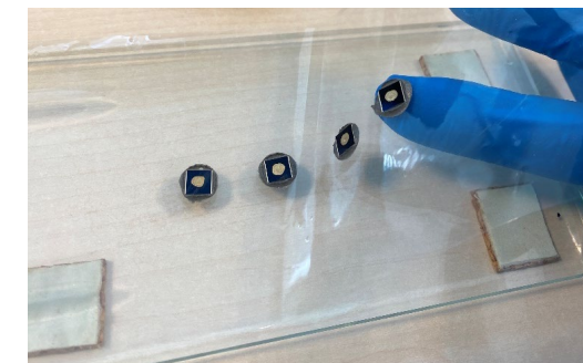
Solder paste deposition jig and Teflon film for safe cell handling
