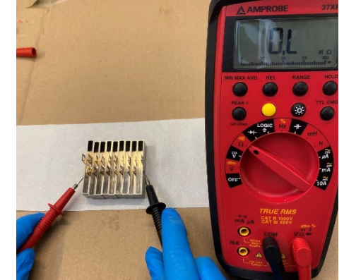
Varnish inspection under UVA light and electrical test
