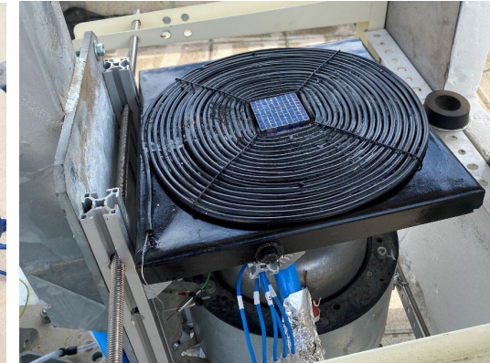
CPV dense-array of 9×9 CPV cells, the DC/DC converters and the perimetral thermal absorber
