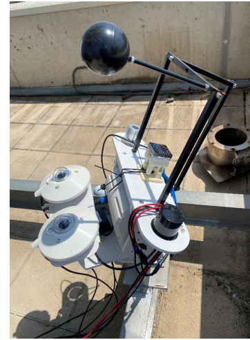
TEK3000 S10 automatic solar tracker pyrheliometer
