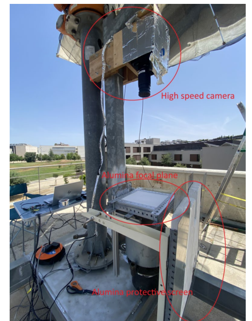
Experimental setup for optical flux characterization
