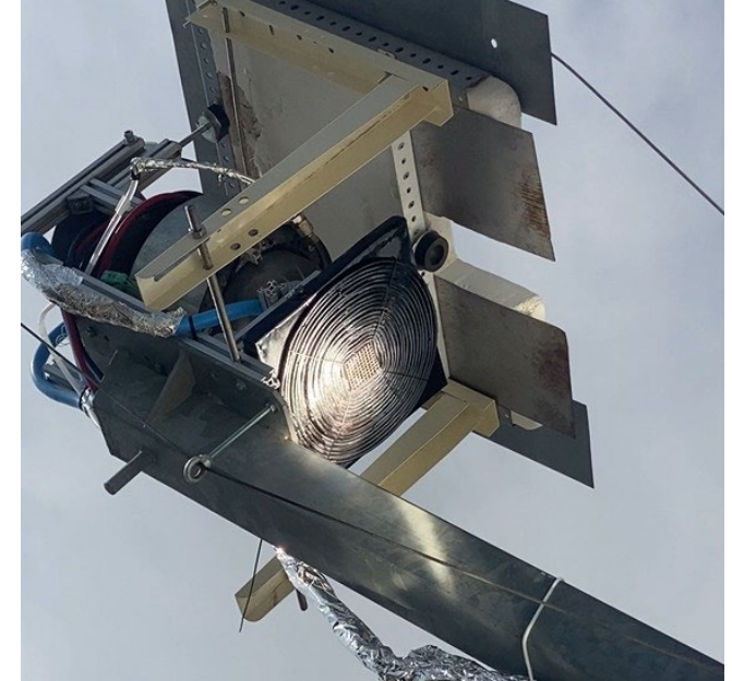
CPV receiver in operation at dish focus
